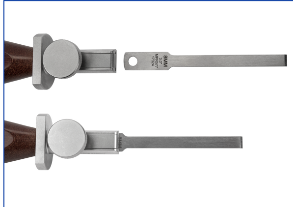
Figure 4 | With assembly loosened, insert the mating end of the blade into the slot until fully seated. Tighten, and test to ensure blade is secure.
